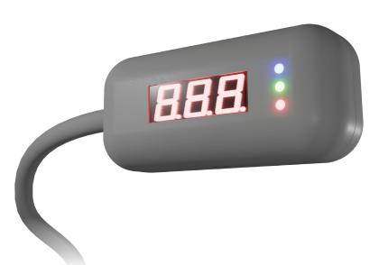
OCTOPUS is a bus interface allowing the interaction between OVER Building Energy Management System (BEMS) with generic devices like digital/analog sensors, dry and voltage contacts. OCTOPUS is designed with a main electronic base that can be plugged with interchangeble specific interfaces, each one with different features.
