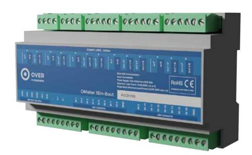
Device for measuring energy consumption (active and reactive), for single-phase lines (230Vac 50Hz) able to control the electrical power status of connected loads such as lights, sockets, shutters, timed lights, etc. The device has 16 programmable digital inputs to which buttons, switches, sensors or alarms are possible to connect. These inputs can be useful for controlling the on/off status of the power outputs of the same OMeter or any other device connected to the same BUS.
